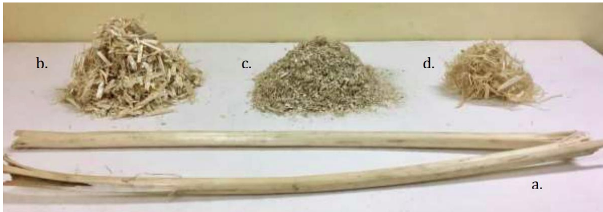
Slika 2: a. konopljino steblo; b. zmleto konopljino steblo; c. pezdir; d. konopljiona (vir: Jami, Tarun & Karade, Sukhdeo & Singh, L P. (2018). Hemp Concrete – A Traditional and Novel Green Building Material)
